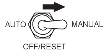
Figure 42. MPEC Control Switch (Manual Position)
